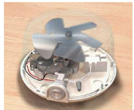
Above Left A 1960s advert for the Sleep-Mate. Above Right Buckwalter's 1964 patent. Right The fan inside a Dohm.
